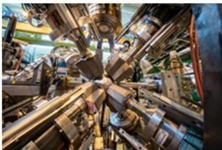
The highly-segmented MINIBALL high-purity Ge-detector array coupled to the HIE-ISOLDE post-accelerator.
