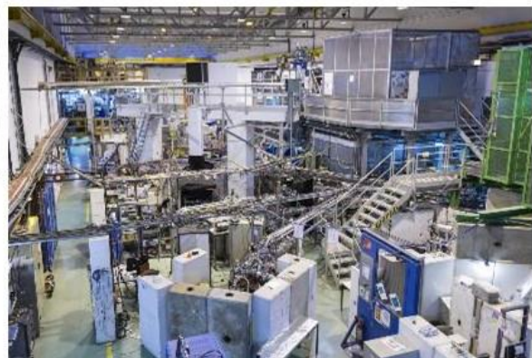
The highly-segmented MINIBALL high-purity Ge-detector array coupled to the HIE-ISOLDE post-accelerator.
